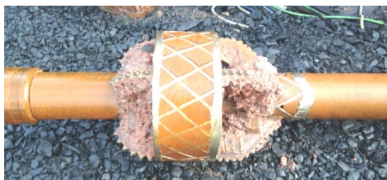
Figure 16. Typical flycutter hole opener
